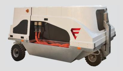
The diesel engine driven GPU is designed to reduce CO2 emissions with its technical characteristics. The unit can also provide an additional output of standard voltage at The unit is able to operate from the mains, 380-400V, 3 phase main power supply grid as GPU, without fuel consumption.
