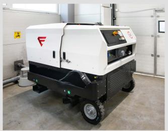
The Hybrid Diesel engine driven GPU is designed to reduce CO<sub>2</sub> emissions with its advanced technical features and optional hybrid configuration.
