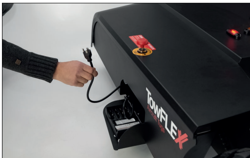
Battery Charger TF3
