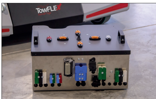
The e-Cube is the Heart of the TF5 Aircraft Tug
