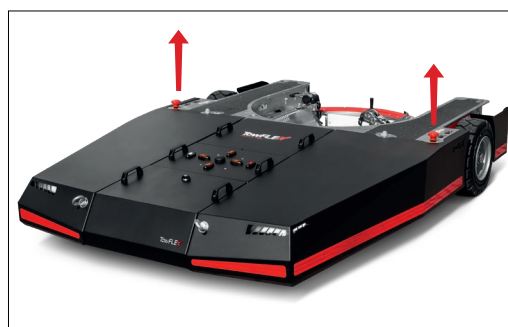
Activate Charger: key switch to off, pull BOTH eStops up
